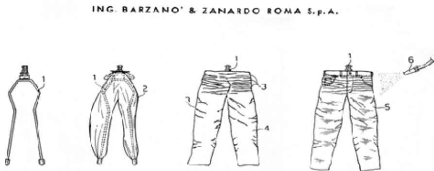
Fig.4 – Production stages in the ageing of blue jeans that are sandblasted after being placed on a mannequin.
