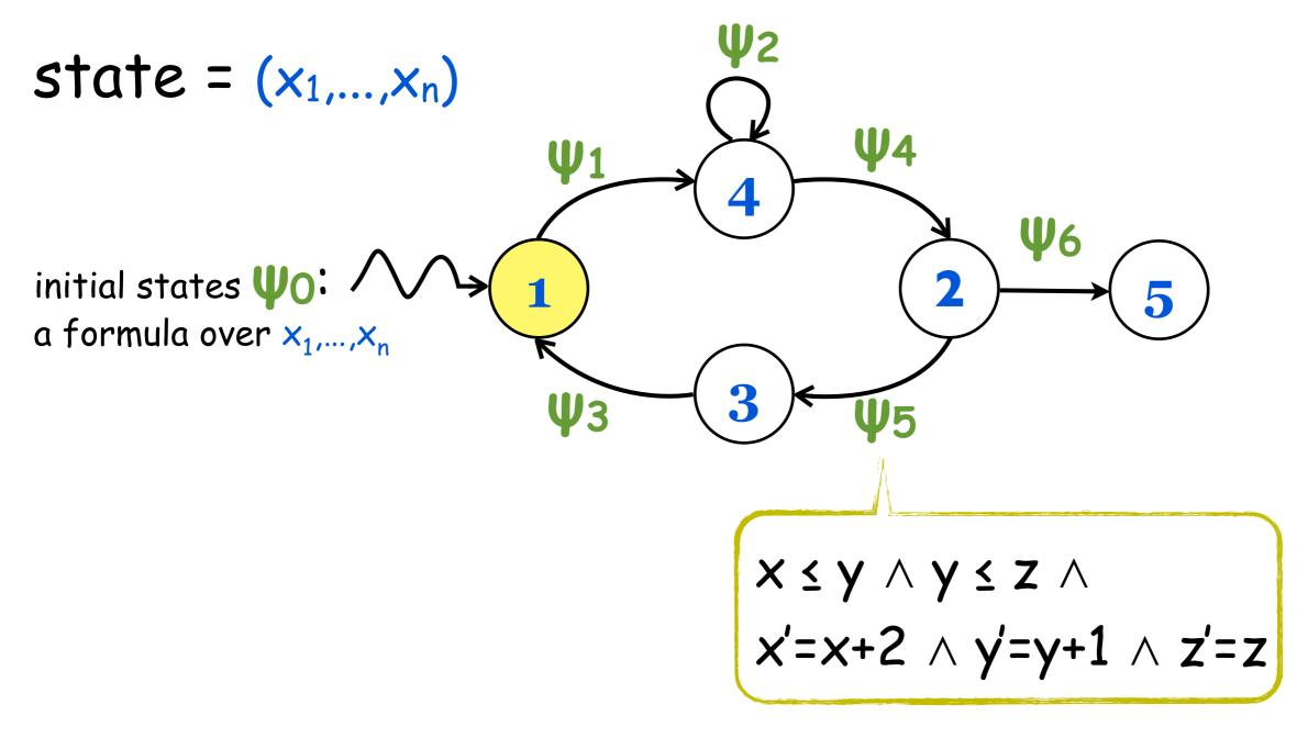
$\psi_i$  are conjunctions of linear constraints over the variables  $x_1,...,x_n,x_1',...,x_n'$
